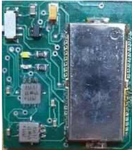
Figure 1 – Laboratory prototype of the wireless unit for the vibration diagnostics system for power equipment
