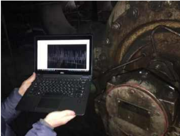
Figure 2 – Functionality testing of a laboratory prototype of a wireless vibration diagnostics system for power generation equipment at the Darnytsia CHP
